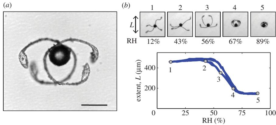
**Figure 1.** (a) The four elaters of a spore unfurling in a dry atmosphere. Scale bar, 50  $\mu\text{m}$ . (b) Elater extent as a function of the RH. Curves obtained by varying the humidity at a rate of 1% RH per minute. Circles 1–5 on the curve correspond to the five pictures. (Online version in colour.)
