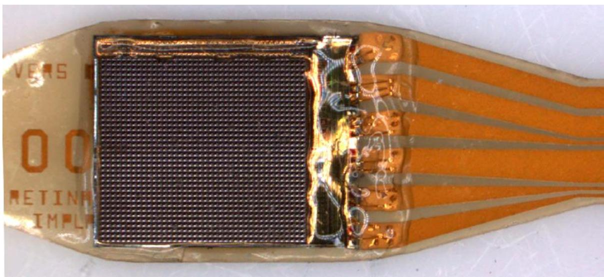
**Figure S2:** Magnification of the vision chip with 1500 photodiodes, amplifiers and electrodes. The bonding points connect the chip to the gold wires for power and signal transmission, positioned onto the subretinal foil that leaves the eye through a scleral flap close to the equator of the eye bulb.
