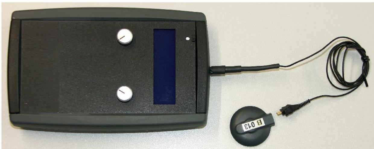
**Figure S3:** Handheld unit for power supply and adjustment. The user can adjust the contrast sensitivity and gain using the two knobs. The handheld unit is connected to the implant by an electromagnetic coil that is magnetically held in position over the retroauricular secondary coil.
